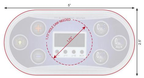
Once ready to install, plug one end of the topside cable into the back of the T7-S, snake the cable through the cutout in the shell and down to the control box, and plug the opposite end of the topside cable into the control box. Affix the topside by peeling off the paper over the adhesive tape on the back of the topside, than pressing it firmly into place, slowly pressing firmly all around the perimeter to assure a good bond to the shell.
