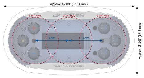
Once ready to install, plug one end of the topside cable into the back of the T8-S, snake the cable through the cutout in the shell and down to the control box, and plug the opposite end of the topside cable into the control box. Affix the topside by peeling off the paper over the adhesive tape on the back of the topside, than pressing it firmly into place, slowly pressing firmly all around the perimeter to assure a good bond to the shell.
